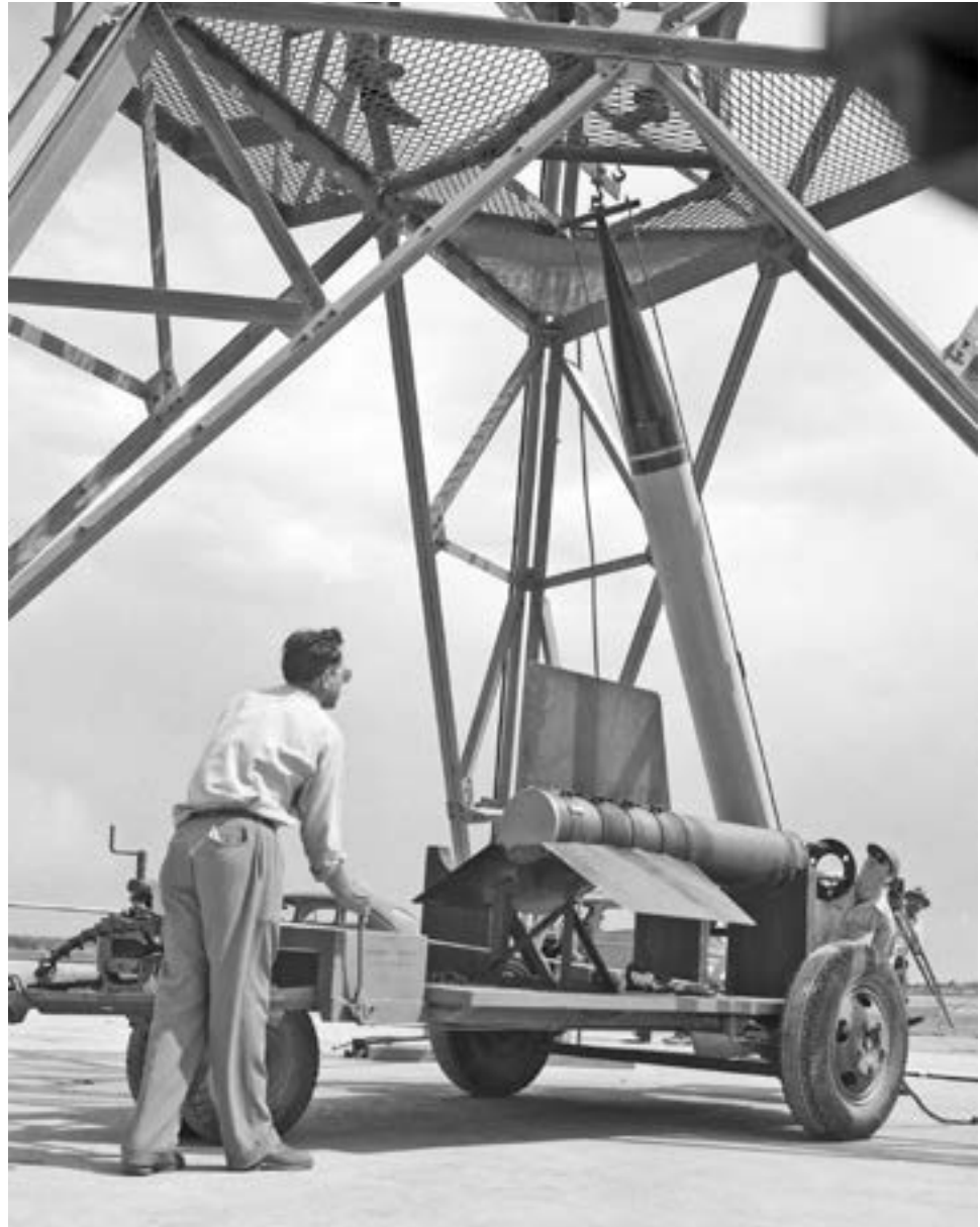
A WAC Corporal rocket, almost erect with the black nose, is being loaded into its launch tower at the Army Launch Area by engineers from the Jet Propulsion Laboratory (JPL), date unknown. Laying on the trailer, with the large fins, is the Tiny Tim booster used to accelerate the rocket to a high enough speed, it will be stable as it leaves the 100-foot tower. James M. Flanagan papers. Ms 0259. New Mexico State University Library, Archives and Special Collections Department.
