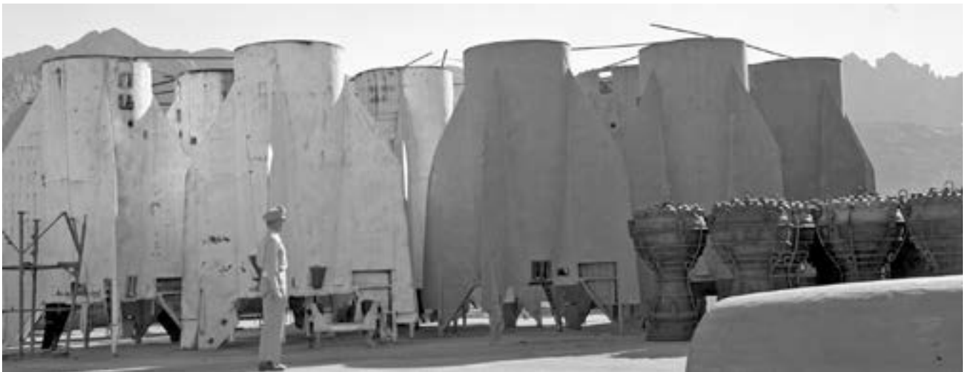
Some of the V-2 rocket tails and rocket motors stored outside the old hanger used for rocket assembly, date unknown. The material was all trucked over San Augustin Pass from the railyard in Las Cruces. Flanagan’s escort provides some scale. James M. Flanagan papers. Ms 0259. New Mexico State University Library, Archives and Special Collections Department.
