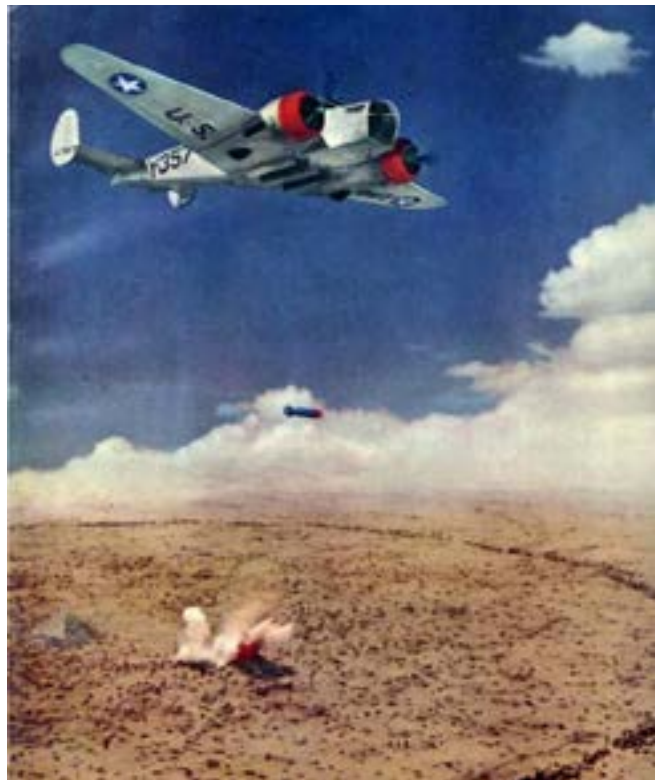
Beech AT-11 dropping sand-filled bombs at target. (Image courtesy of Creative Commons, Army Air Forces Collection, Deming Army Air Field 1943-12 Class book.)
