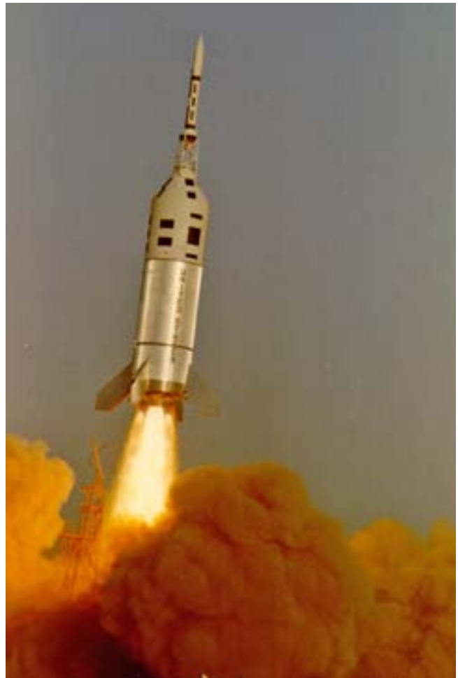
The first test of the escape system using the Little Joe II vehicle on May 13, 1964. (White Sands Missile Range Museum photo.)
