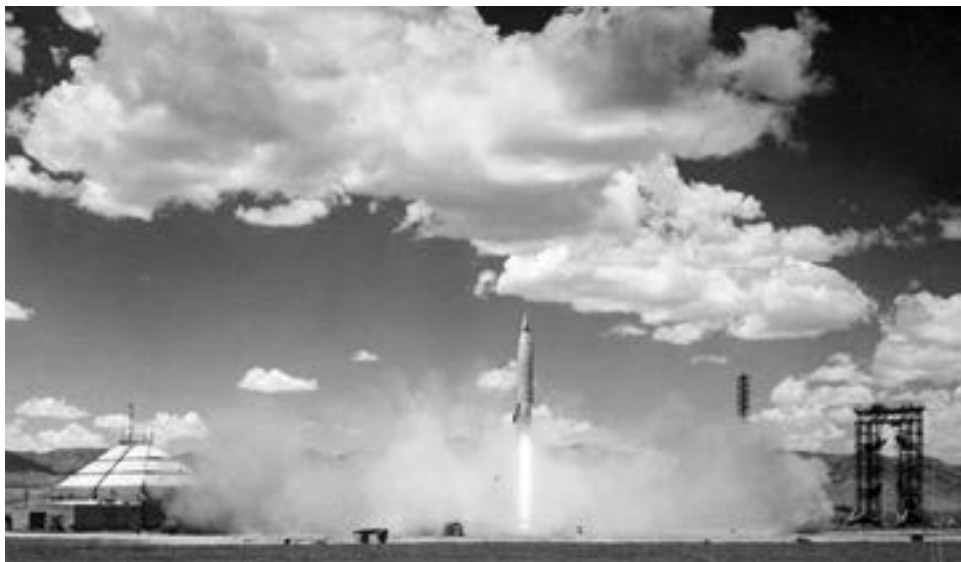
This typical V-2 launch was on July 10, 1947 from Launch Complex 33, now a National Historic Landmark. On the left is the Army blockhouse used to protect men and equipment during launches. On the right is the V-2 gantry used to erect the rockets and prepare them for flight. (White Sands Missile Range photo.)
