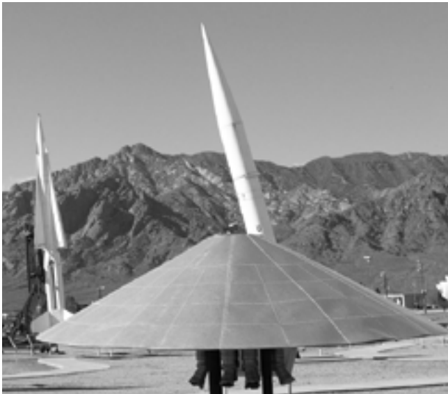
The PEPP Aeroshell on display at the White Sands Museum is often jokingly referred to as the missile range's flying saucer. Below the saucer are the small rocket motors used to propel it to supersonic speeds. (White Sands photo.)
