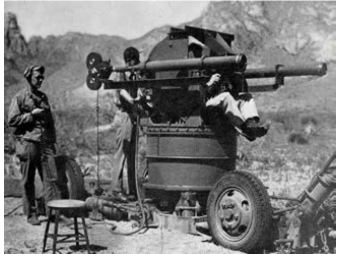
First prototype tracking telescope known as Little Bright Eyes or T-1. This picture was taken at F-Star site, located at the foot of the San Andres Mountains. Clyde Tombaugh is at the controls. US Army photo.
