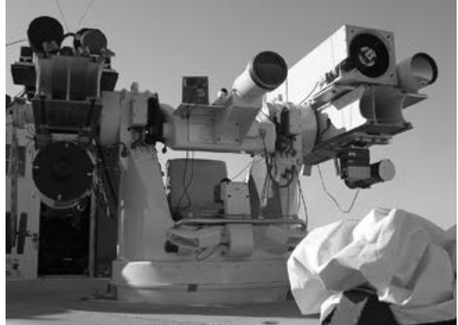
Kineto Telescope Mount or KTM is the tracking system utilized presently at WSMR and at Kennedy Space Center for mounting various high-resolution cameras. Photo by Bill Godby
