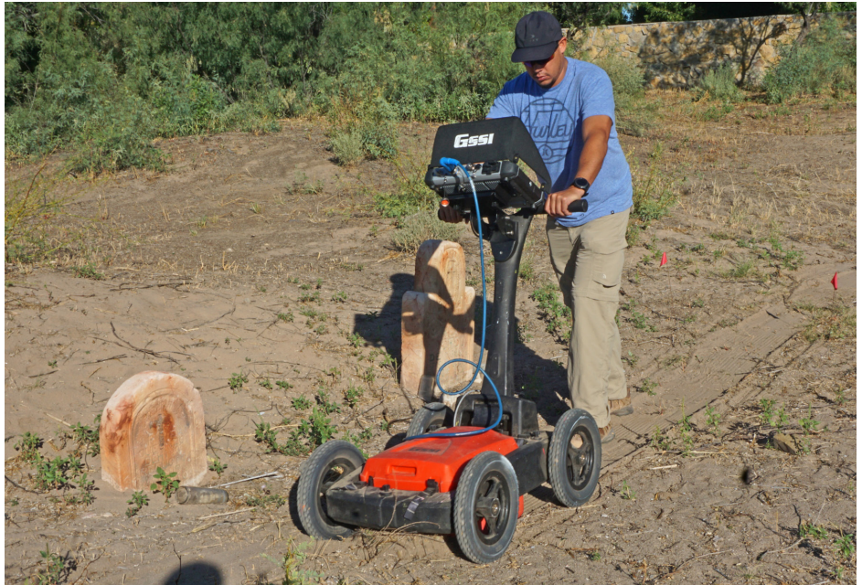
CSTi employee David Acosta, from the Las Cruces office, runs the company's ground penetrating radar over the old Picacho cemetery.
