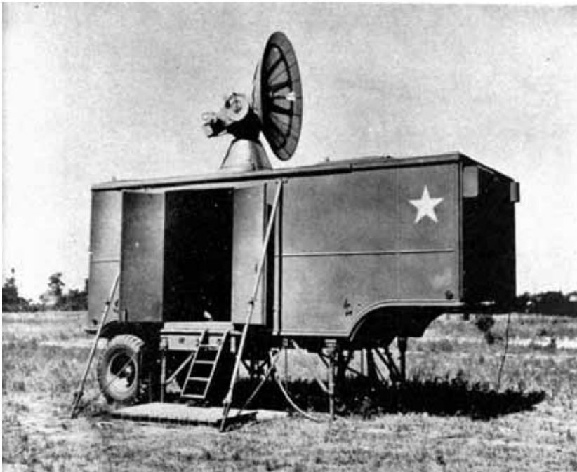
An early SCR-584 radar with the dish mounted atop a trailer. This was the configuration used early on at White Sands Proving Ground to track V-2 launches. From the author's collection.
