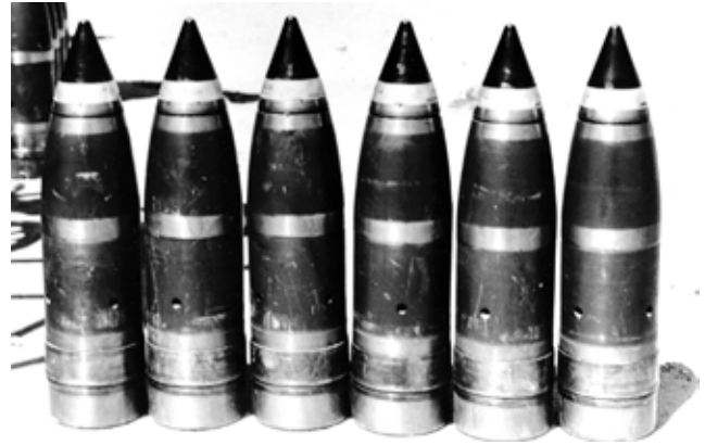
The photo above shows artillery shells equipped with proximity fuzes. The photo below shows a recovered fuze after firing. The fuze was created before the digital age and is remarkably small for its time - that is a dime in the foreground. From the author's collection.
