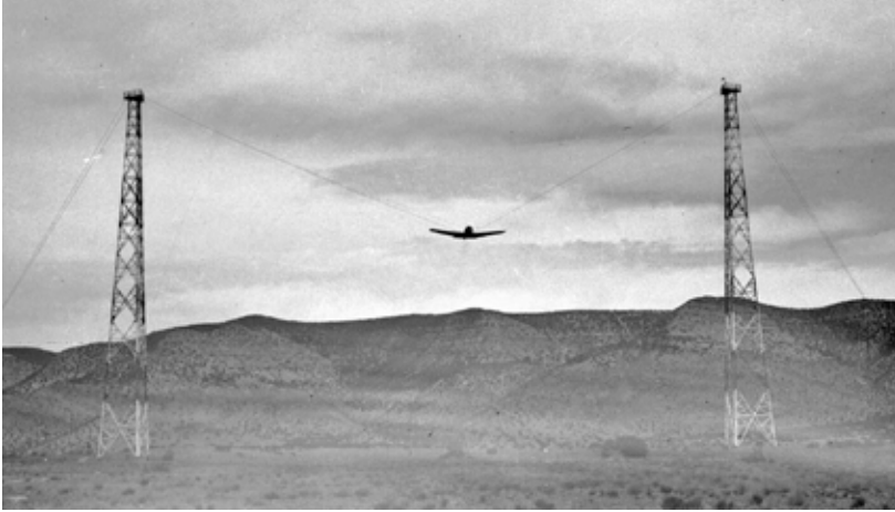
The two towers erected at the test facility with an aircraft mockup suspended by rope between them. From the author's collection.
